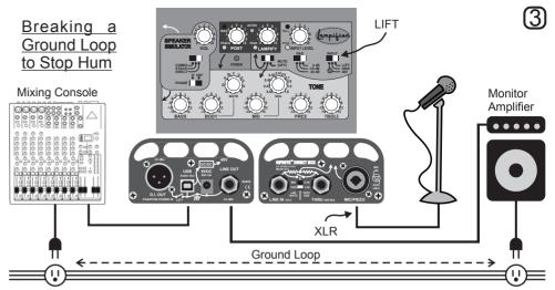
Eliminate an annoying ground loop between mixer, amp, computer, etc.
