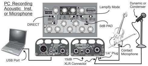
Make high-quality digital recordings of any audio source plugged into the direct box. Connect directly to your computer using the included cable.
