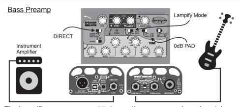
The Lampifier processor provided smooth response and good sustain. Add a contact mic or piezo pickup to use this setup for string bass instead.
