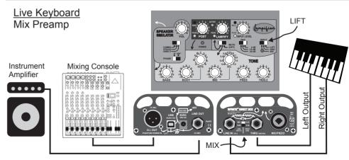
Mix left/right channels for live performance while breaking a ground loop.
