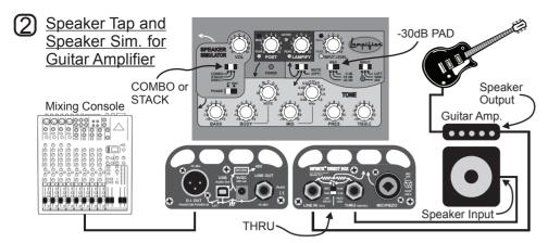
Captures the sound of a guitar amp without a mic. The direct box taps the speaker output and simulates a speaker cabinet for the D.I. Output.
